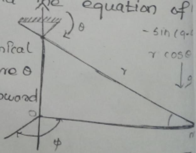
The angle  $\phi$  is measured between a vertical reference plane passing through the vertical axis.
