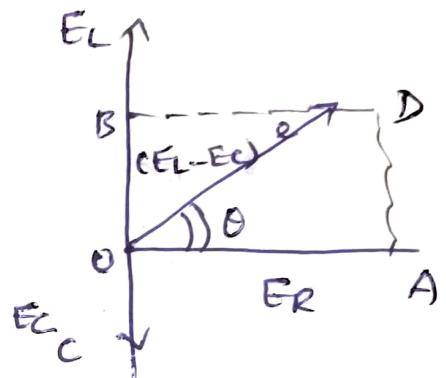
$\Rightarrow$  The voltage drop across the resistance is in phase with the current, the voltage drop across the inductance is leading the current by a phase angle  $\pi/2$  and the voltage drop across the capacitance is lagging the current by a phase angle  $\pi/2$
