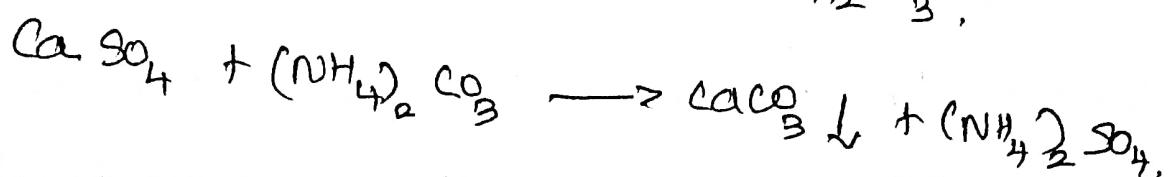
\* The precipitated  $\text{CaCO}_3$  is filtered off. The filtrate is concentrated by evaporation under vacuum. On cooling, crystals of  $(\text{NH}_4)_2\text{SO}_4$  are got. The crystals are dried, packed and sold under the name Sindri fertilizer.
