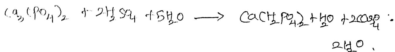
The solid product including gypsum is crushed to a fine powder and sent for direct use or mixed with Nitrogen and Potash fertilizers to make NPK fertilizer.
